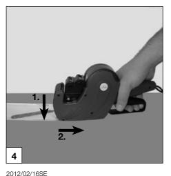
Place the printer onto the correct location and pull slowly and carefully to the rear (towards you).
