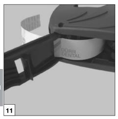
• Pull the label end through front slit in the lower cover.
